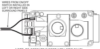
NOTE: TO OPERATE INSERT WITH SIDE PANEL ON/OFF SWITCH, BE SURE TO PLACE THE MAIN SWITCH (TO THE RIGHT SIDE OF GAS VALVE) TO "**OFF**" POSITION.
